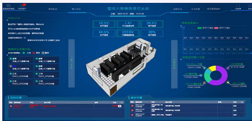
Figure 2.5-2 real-time temperature and humidity monitoring, power monitoring, and PUE (Power Usage Effectiveness)
